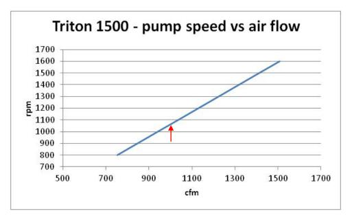
Let's say for example, that a client wants to target 1000 cfm airflow. This chart says that he'd need to turn the pump at ~1050 rpm to obtain that volume of air. (As mentioned, this is under
